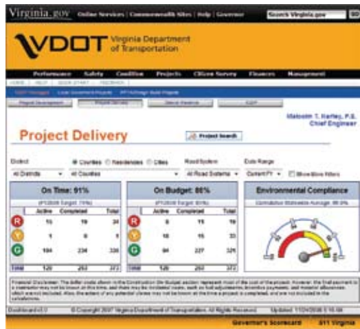
Figure 1: This VDOT dashboard screenshot lays out a series of gauges showing KPIs for highway performance, safety, condition, projects, financing and operations.
